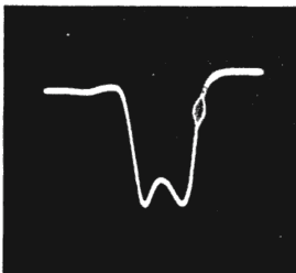
Figure 7-J Overall video IF response curve cor- rected by retuning last stage. Birdie at 26.4 mc.
