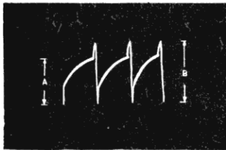
Vertical Saw Gen Grid Tube V16 Pin 4 A - 245 volts B - 290 volts
