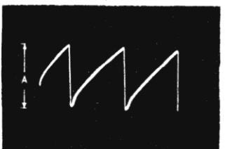
Red and Black Lead on Deflection Coil A - 25 volts
