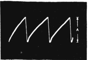
Horizontal Saw Gen Plate Tube V18 Pin 5 A - 50 volts
