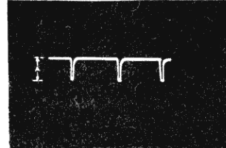
Sync Separator Plate Tube V15 Pin 2 A 7.5 volts
