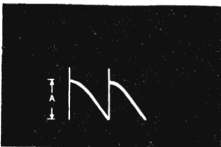
Vertical Deflection Amp Tube V17 Pin 2 Flat portion on upper part of curve due to extreme position of linearity control A 125 volts
